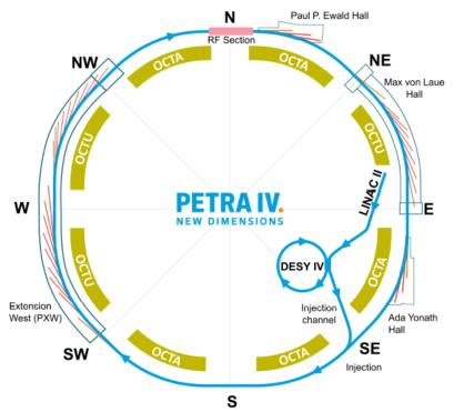
The storage ring will feed up to **30 undulator** insertions (photon beam can be further split to allow more experimental stations). <u>Ultra low emittances</u> in the region of 10 pm.
