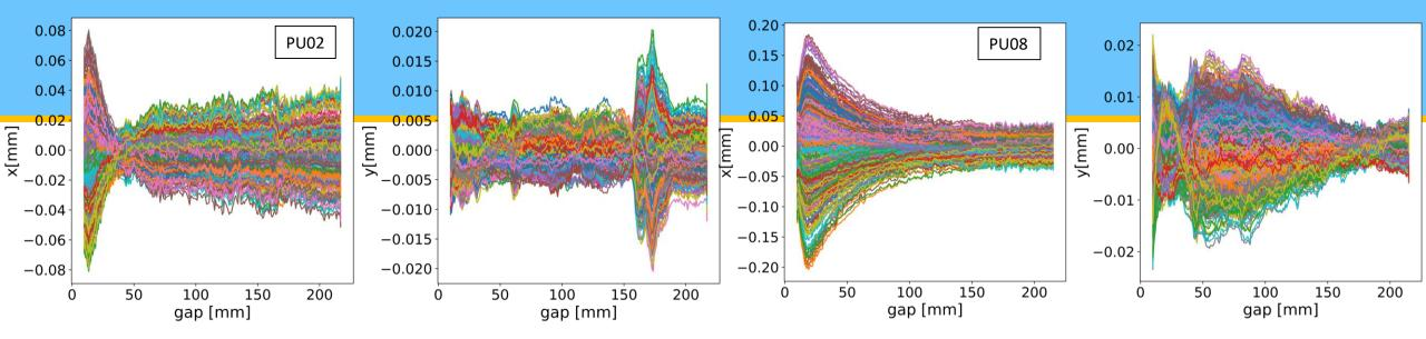
Measurements of the horizontal and vertical orbit were taken varying the gap size in their operation range for 18 IDs in PETRA III. Each colour represents a BPM along the ring.
